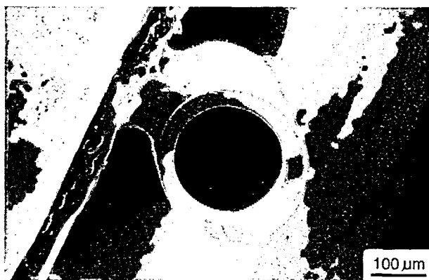
FIG. 7 SEM photograph of the glass capillary membrane.
